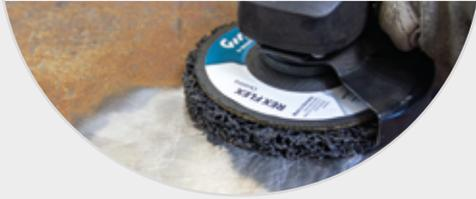
**Cleaning and preparing material surface** by removing rust, scale or paint from the surface. Does not remove the base material. REX is available in many different forms.
