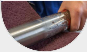
**Abrasive grain, is embedded in a 3-dimensional nylon web.**
