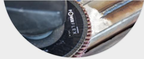
**Material removal, weld seam processing, matting or structuring** – a wide variety of grinding materials tailored to every application. A selection of premium abrasive grains on a cotton, polyester or poly-cotton backing.
